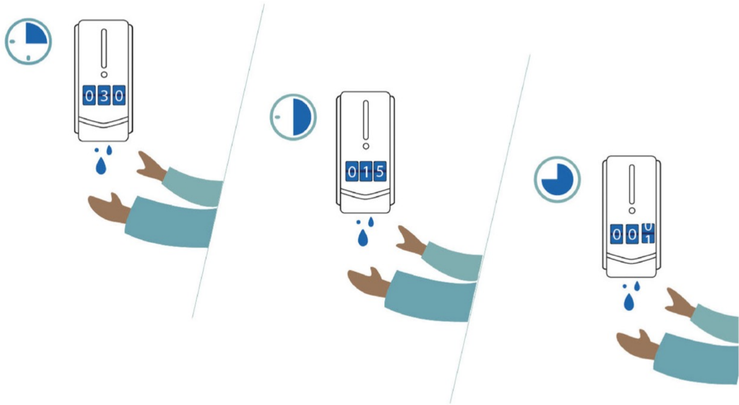
Figure 3. Gel dispenser redesign: a gel dispenser than counts down when used to give an indication of normal daily use.
